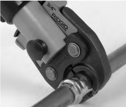
Figure 7 – Placing Scissor-Style Jaws Around Fitting
