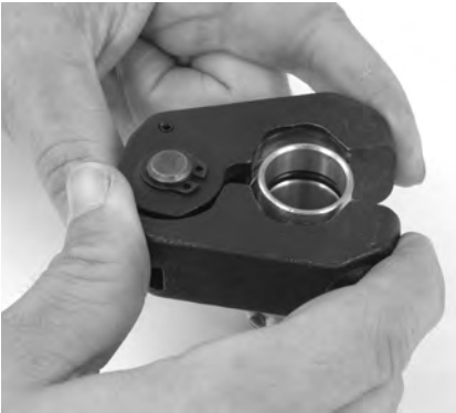
Figure 9 – Installing Press Ring onto Fitting
