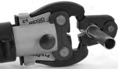
Figure 10 – Attaching Actuator to Press Ring
